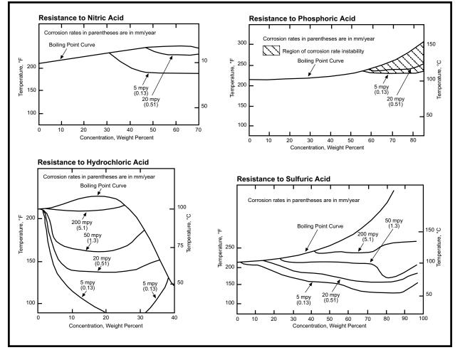
\*All test specimens were heat-treated at 2050°F (1121°C), rapid quenched and in the unwelded condition.
