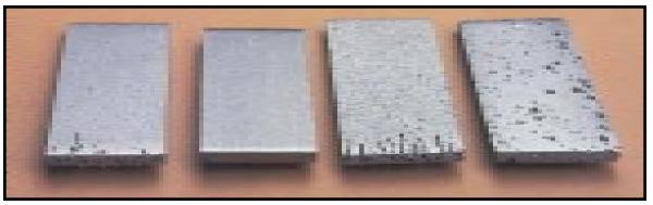
Samples were subjected to a solution of 11.5%  $H_2S0_4,$  1.2% HCl, 1% FeCl<sub>3</sub> AND 1% CuCl<sub>2</sub>. Solutions for coupons 625 and C-4 were at 102°C, while C-276 and C-22 were at 125°C.
